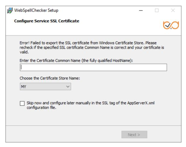
You can either try to type the certificate common name and select a proper Certificate Store Name or skip this option and provide the information later using the SSL tag values of the AppServerX.xml file.
