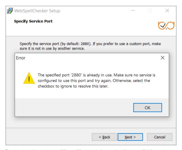
To continue the installation under the port 2880, press **OK** and select the **Ignore and use this port even if it is in use** option.
